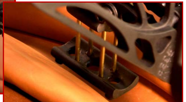
BALANCE BEAM IN CENTER OF GULLET CREATES A "Z" AXIS REFERENCE
